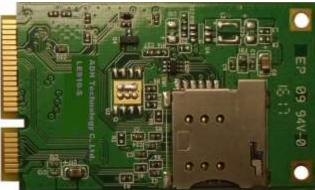
LE910-S is a versatile and easy-to-use 4G Cat 1.0 device that provides LTE capability, easy to integrated into devices or application systems. It creates new opportunities to design device smaller and efficiently. It is the latest step towards true wireless intelligence from the world leader in mobile solutions.
